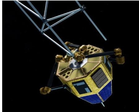
*Figure 4: The Archinaut: ULISSES 3D printing and assembling a boom structure [4]*
