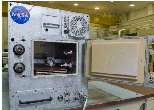
*Figure 6: TUI's Refabricator, capable of printing and recycling print material [8]*
