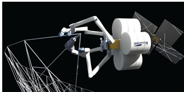
*Figure 5: Rendering of TUI's SpiderFab printing truss structures for large dish [6]*
